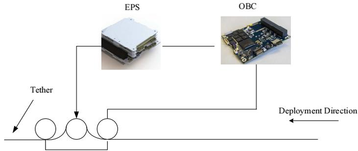
Figure 3. Circuit for measuring tether length
