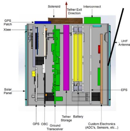
Figure 1. Top Level Block Diagram of Daughter Satellite
