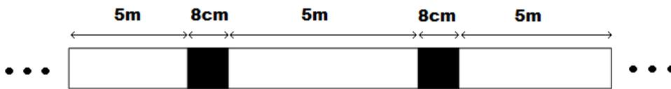
Figure 4. Coated tether segments (8cm long) with intervals at every 5m
