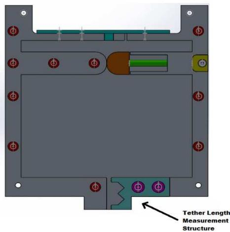
Figure 2. CAD model of tether storage box
