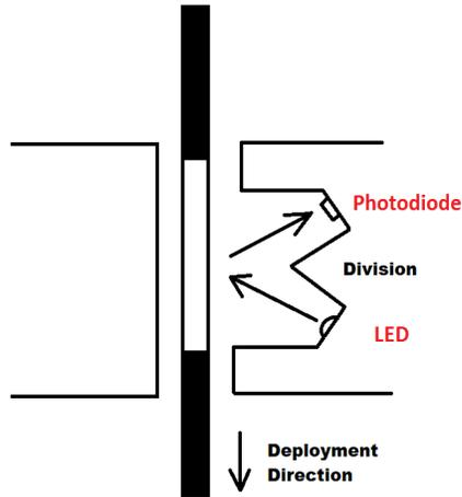
Figure 6. Placement of the LED and photodiode alongside the divider
