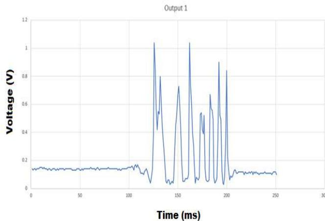
Figure 7. Spikes suggesting the reflected portions of the tether
