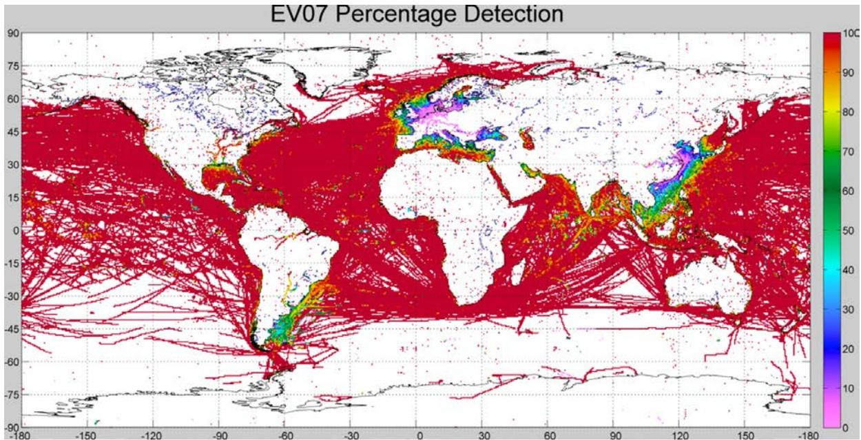
**Figure 4: Estimated Vessel Detection Rate (Percentage) for M3MSat (EV07)**
