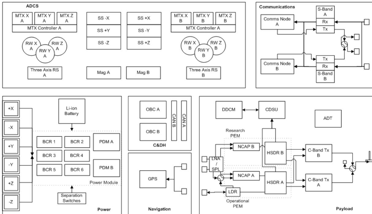
**Figure 2: M3MSat Simplified Spacecraft Block Diagram**
