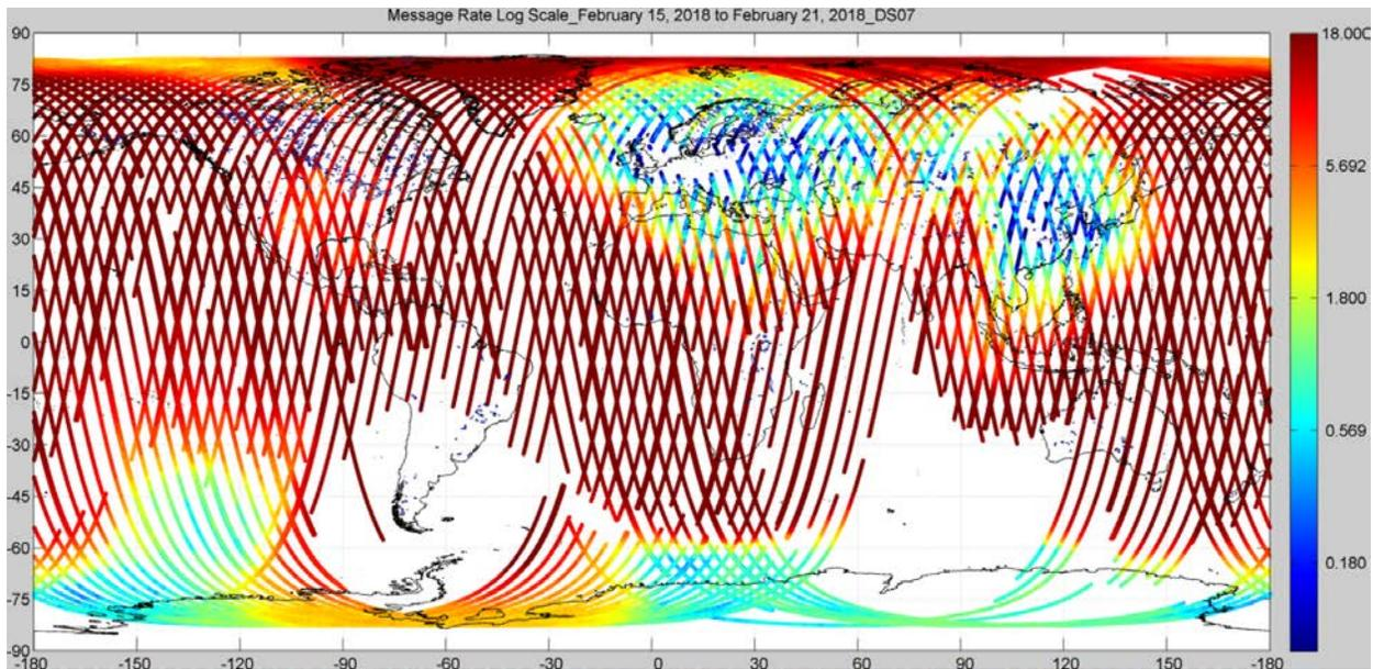
**Figure 3: Messages per Second detected by M3MSat from February 15 to 21, 2018**
