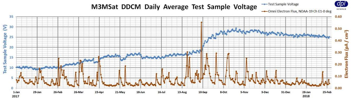
**Figure 5: DDCM Daily Average Test Sample Voltage (courtesy DPL Science Inc.)**
