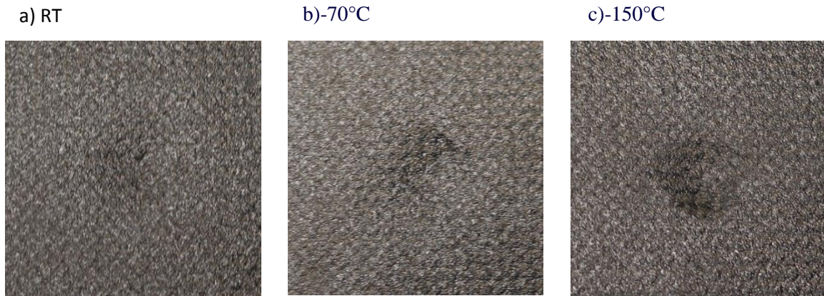
Figure 3. Typical damage for specimens impacted with the 25.4 mm diameter impactor and the 10 kg mass.
