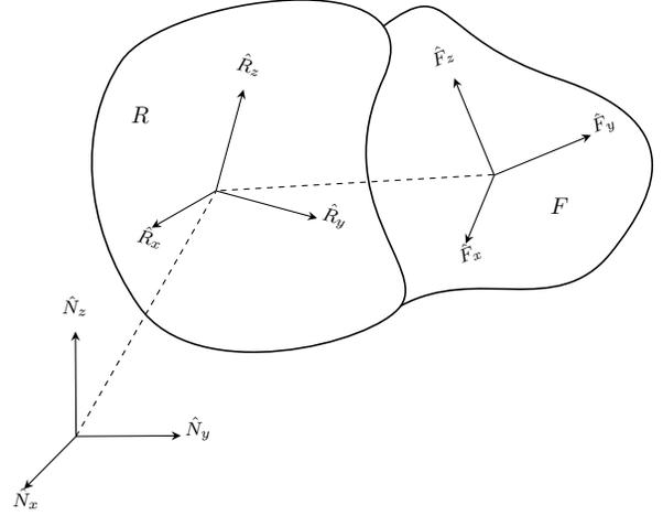
Fig. 1: Rigid body  $R$  and flexible body  $F$ .
