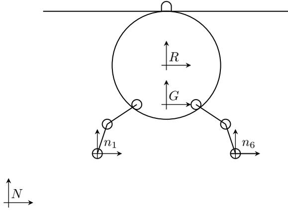
Fig. 4: SRAMSS-2D rigid-flexible aircraft system frame configuration.
