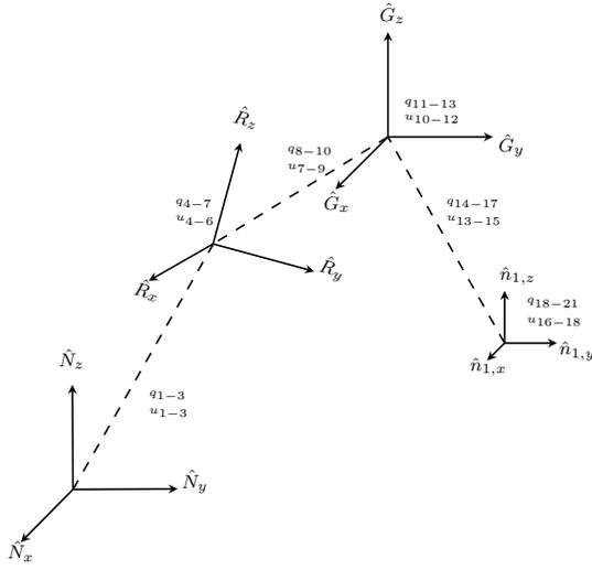
Fig. 3: Generalized coordinates  $\mathbf{q}$  and speeds  $\mathbf{u}$ . Each frame is described relative to the previous frame in the chain by a pair of translational and angular vectors containing generalized coordinates and speeds. In this figure, only the open chain branch to frame  $n_1$  is shown for clarity.
