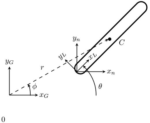
Fig. 5: Planar beam coordinate systems.
