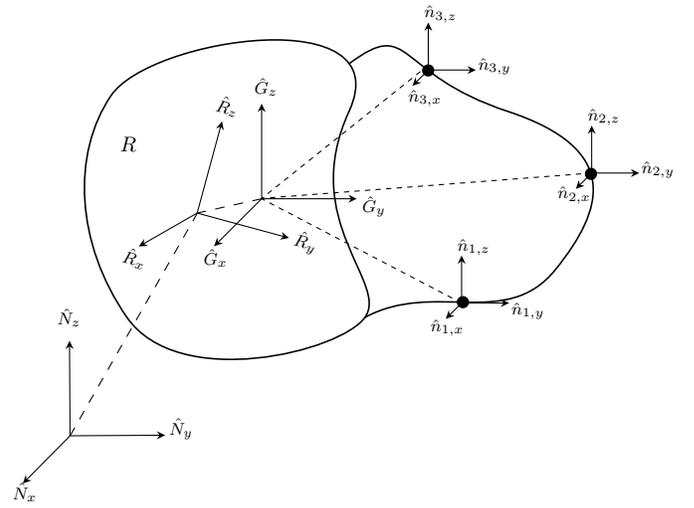
Fig. 2: Rigid-flexible body frames of reference. The generic body in this figure is considered to have a three-node finite element representation.
