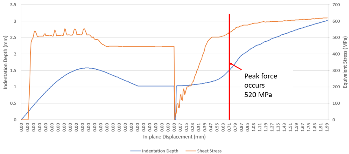
Figure 8: Indentation depth (blue) and Equivalent stress (orange) curves versus panel displacement during compression, for the simulation with no residual stress.
