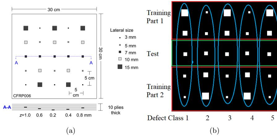
Figure 2: (a) Scheme of the specimen used for the experiments and the specification of the holes, (b) Train and test split.
