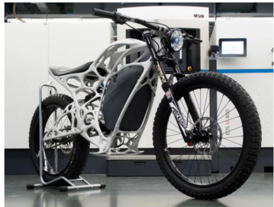
Figure 1: Airbus Light Rider manufactured with AM in separate components [4].
