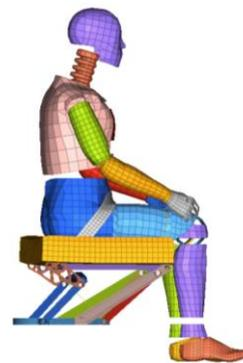
Figure 2: FEA model of the 50% Male ATD on the preliminary seat structure design
