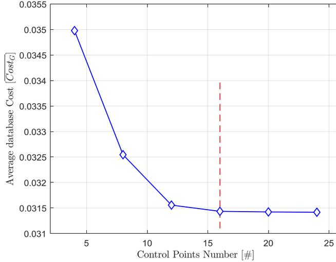
**Figure 3. Graphic showing convergence of the average of the geometrical  $\overline{Cost}_G$  according to the number of control points**
