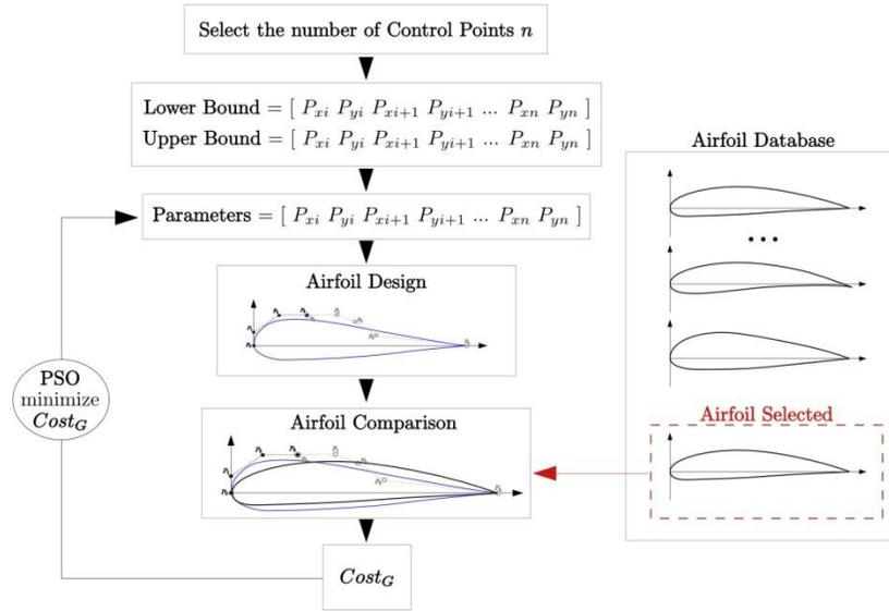
**Figure. 2 Process that was used to find how many control points were required to match with the airfoil database**
