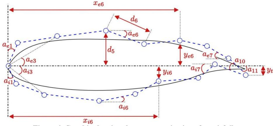
Figure 4. Graphic showing the parameterization of an airfoil using the airfoil generator developed
