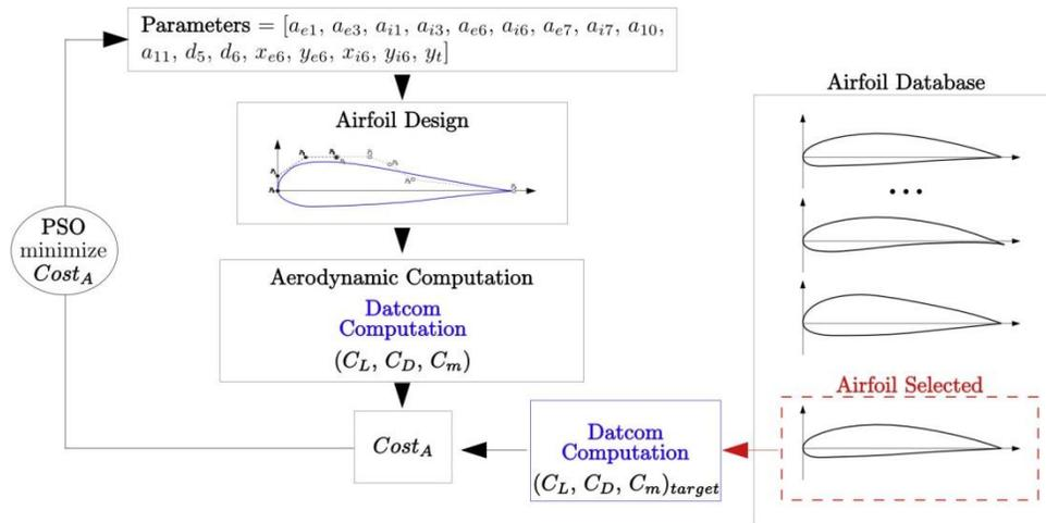
**Figure 7. Representation of the aerodynamic research process**
