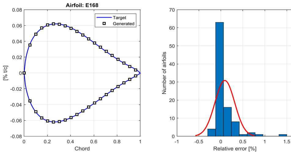
**Figure 6. Results of geometric research for the 88 airfoils of the database**
