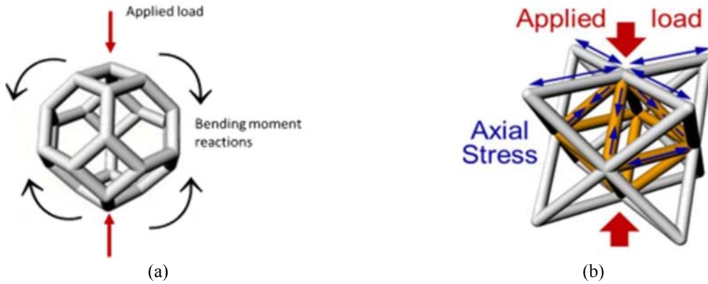
Figure 7: MSDO lattice structure unit cell structure of the (a) Kelvin cell and (b) octet truss [13].
