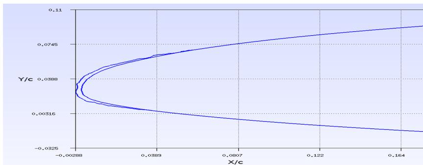
Figure 1: Run Case 606 Iced profile of a NLF-0414 Airfoil
