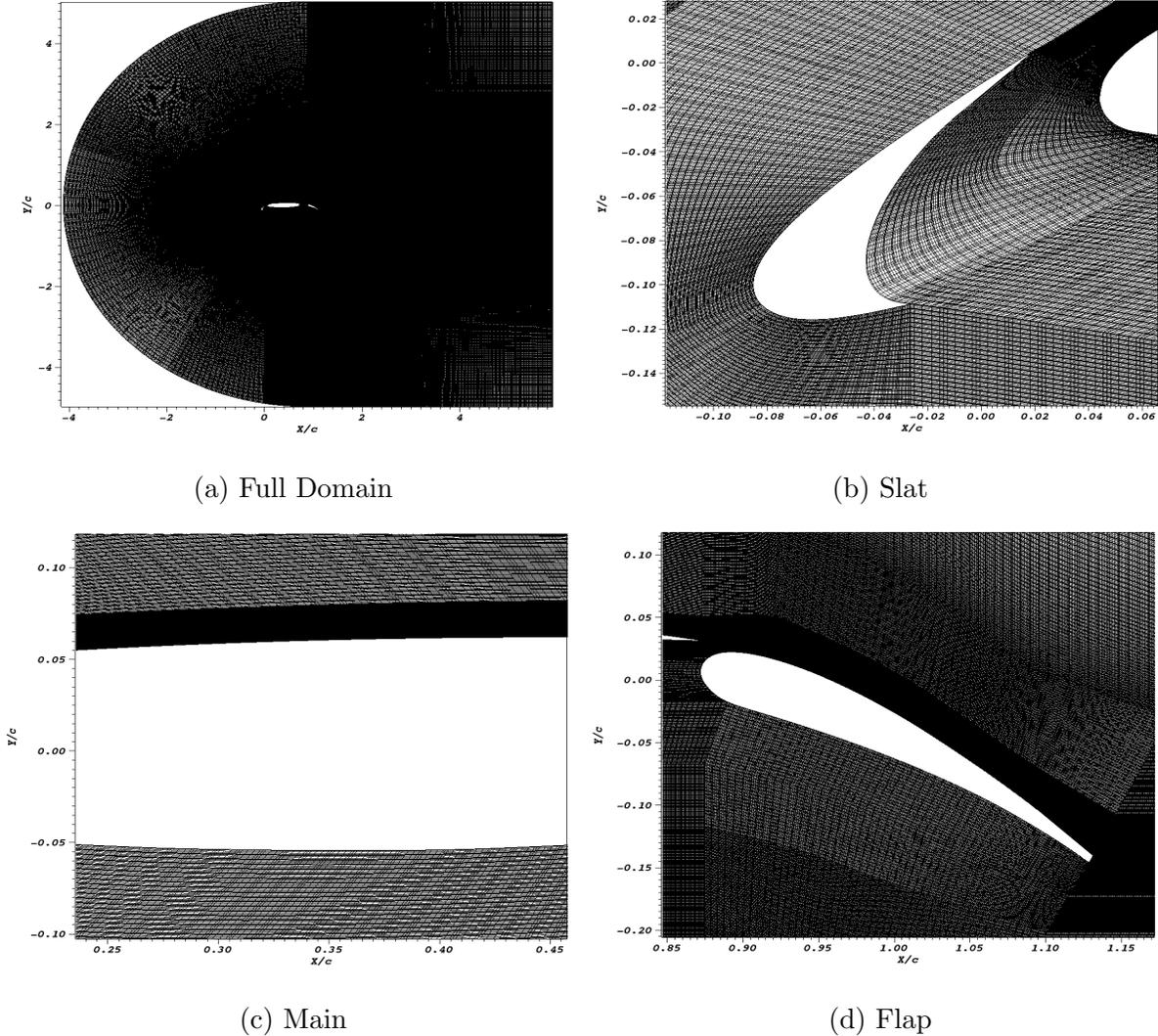
Figure 1: Multi-block spectral element mesh of a 30P30N three-element high lift airfoil
